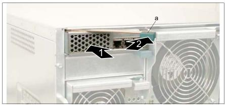
Figure 49: Inserting the I/O blade (a = green touch point)
